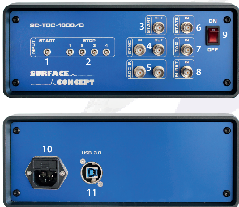
Figure 3: Layout of the SC-TDC-1000 02D R2D8 and R2E8 (similar for R258 but with reduced numbers of inputs and outputs, see below).
